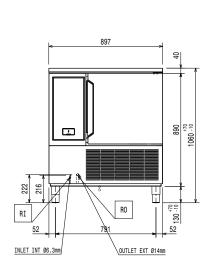
Drain Electrical inlet (power) ΕI Refrigerant Outlet
